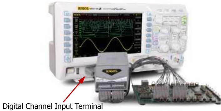
Figure 1-6 To Connect the Logic Probe
